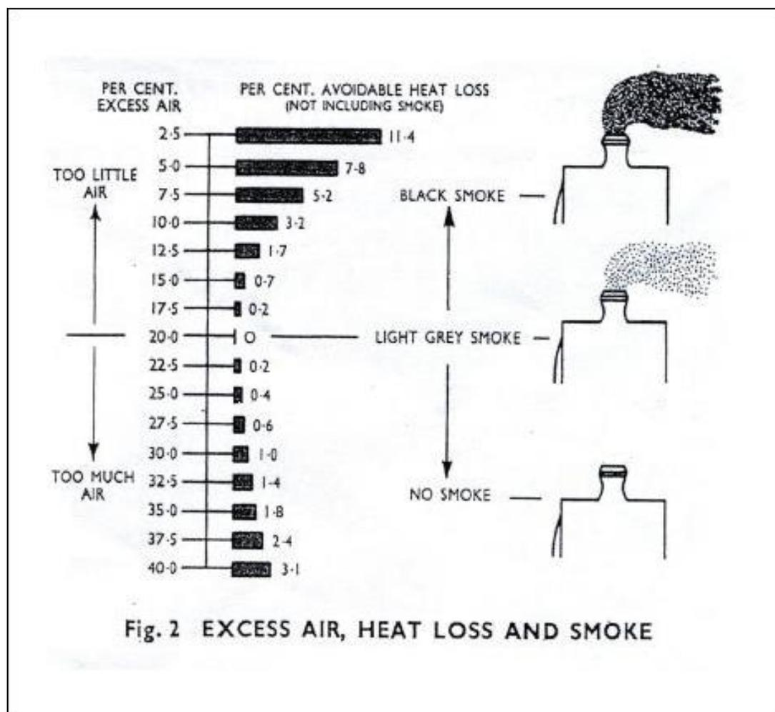
from the fire-bed, together with the larger amount which will be given off immediately the new firing takes place. To obtain the maximum amount of heat for the production of steam, the best method of firing is to limit the
